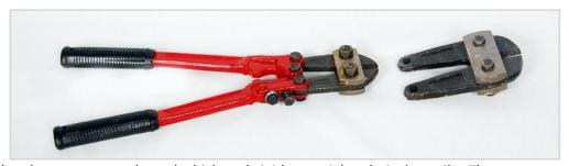
leverage. This enables the user to cut through thick and rigid materials relatively easily. These cutters have adjustable screws for adjusting amount of closure of handles, for blades to make contact with each other. There are two types of Bolt cutters:
