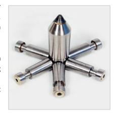
4. <u>Accurate Exit Radii:</u> The exit radii of the nozzles determine the angle of wire exit from one coil to the next. This makes it essential to maintain the exit radii to utmost tolerance limit, which is done using the right calibrating instruments.
